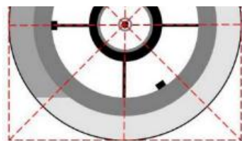
Slow scope collimation - the classic collimation pattern
