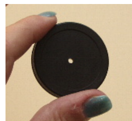
A simple collimation cap
