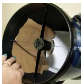
Coloured card applied to scope tube to allow the secondary to be shown more clearly.
