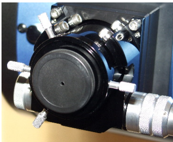
Simple collimation cap on focus tube.
