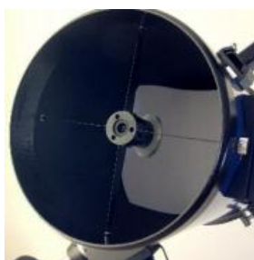
White card inserted into telescope tube to block reflections in the secondary.
