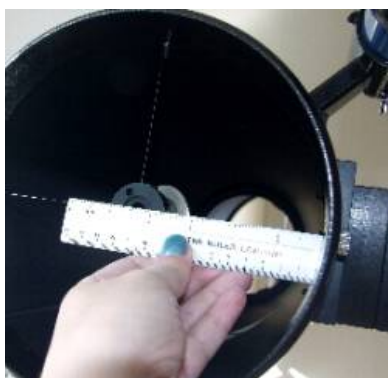
Measuring the spider vanes
