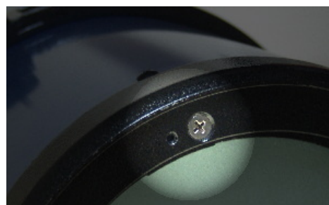
Collimation screws. Lock screw to left, adjuster to right (differs between telescope manufacturers).
