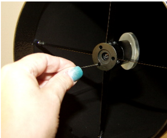
Adjusting the secondary mirrors 'tilt'.
