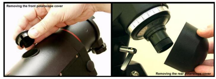
Before starting you will need to remove the covers for the polar scope. The front cover simply clips off, the rear cover has a screw thread. You must also lower the weight bar and rotate the mount through its declination axis until the polar scope is clear. You can check just by looking down the hole underneath the front cover.
