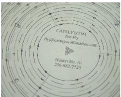
one downloaded from the Catseye Collimation site (www.catseyecollimation.com) and printed it onto a transparent sheet. The template needs to be the same size as the mirror and with its centre marked.
