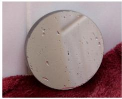
The mirror is now stood up to dry in a warm environment. DO not use a heat dryer or hair dryer. The distilled water if left to dry will not leave any streaks or marks.
