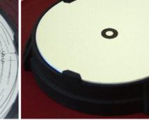
Press the centre of the template lightly and the gently remove it. It should leave the collimation spot physical centre and your ready to reinstall the mirror on the mirror which can be pressed down gently with a cotton bud if need be to get a better adhesion to the mirror surface.
