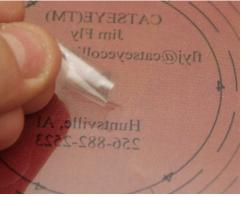
To create a centre spot for collimation you will need. Next you will need a mirror spotting template. I used. Make a small roll of low tack tape or sellotape that's been handled a bit to remove its stickiness and place this onto the template at its centre.
