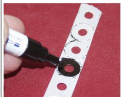
to prepare a spot. I used some hole reinforcers used for filing. These are available from any stationary store. These were blackened using an indelible marker. Let the ink on this thoroughly dry.
