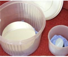
Finally, once fully dry, the mirror is stored in an airtight container and placed on some acid and bleach free paper. The secondary mirror can be treated the same way but DON'T leave it in the water. Some manufacturers will have used a glue to hold the secondary to its mounting which may be affected by water. I prefer to agitate the secondary about in the water rather than just leave it to soak.
