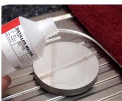
...gently place the mirror in the water and leave it for Now place the mirror on a slightly sloping surface and wash away the soap suds and water using distilled water.
