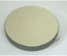
Here is the primary mirror as removed from the telescope in an earlier stage of rebuilding.
